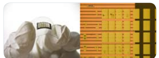
Figure 1. Thin-film transistors fabricated in a strained-Si nanomembrane and transferred to PET. (Courtesy: Haochih Yuan and The Lagally Research Group)
