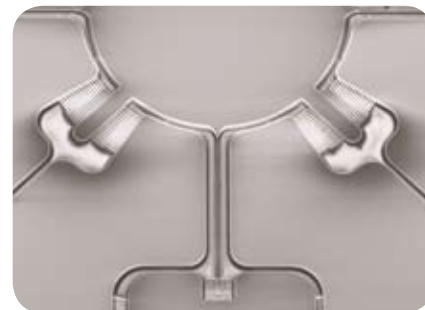
A MEMS optical switch mirror developed using the Micragem fabrication process. (Courtesy: Micralyne)
