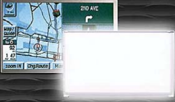
LCD backlight with light guide reduces LEDs.
