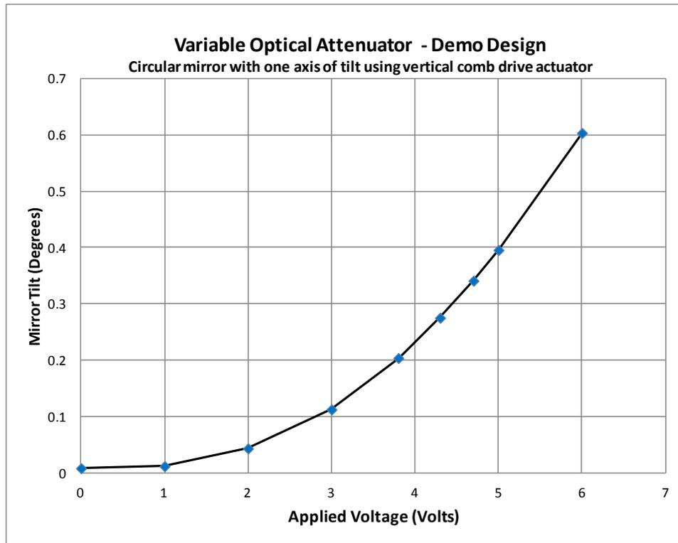
**Figure 4:** MEMS for VOA - Mirror tilt response to an applied voltage
