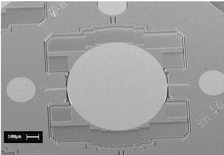
**Figure 3:** SEM Micrograph of the VOA Chip – demo device
