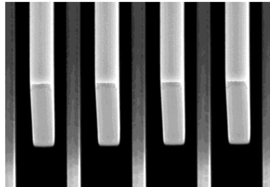
**Figure 1:** Vertical comb drive actuator
